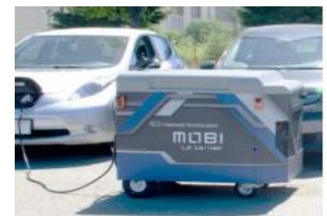
Right: Mobile charging unit to allow for charging away from a chargepoint
